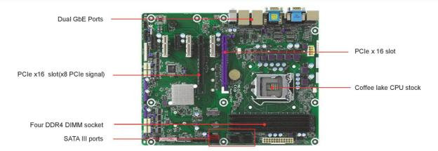
RUBY-D811 is based on Intel® Q370 chipset and Desktop processors including Intel® 8th Gen Core™ i3/i5/i7 SKU. This board supports DDR4 ,PCIe 3.0, and SATAIII. Those fratures help you to build high performance and stabile system.
